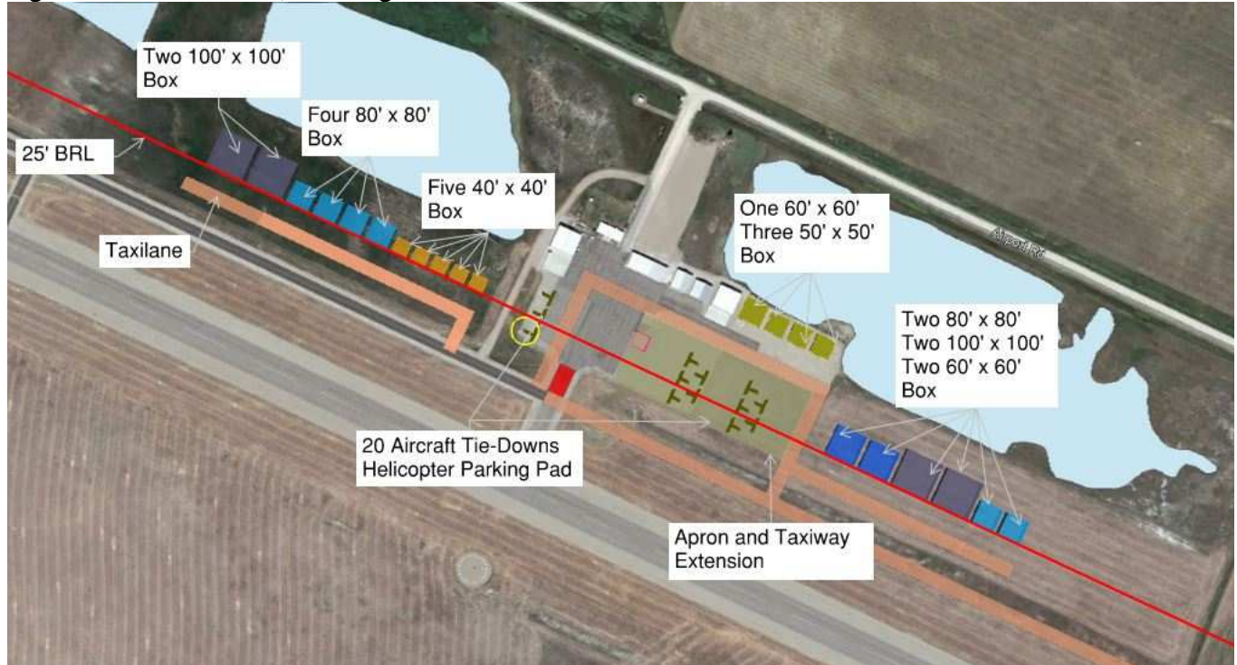
Figure 1.4 Alternative 3, 21 Hangar Facilities
